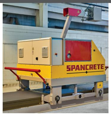
Fully automatic and battery driven, the Spancrete Plotter runs on the casting bed rails and draws all the marks for straight cuts, angle cuts, electrical sockets, slab number, manufacturer logo and different cut-outs on the wet concrete.
